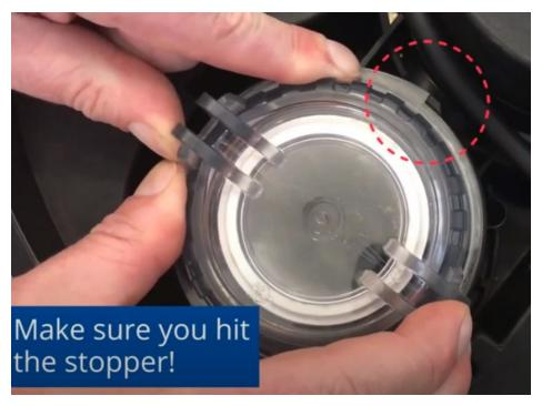
No - Then tighten the cap to the stop.
